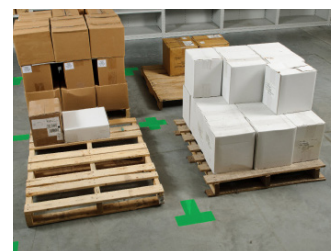
3. Colour-code material storage areas.
